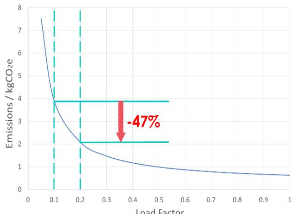
Figure 3 - Emissions against load factor for one of the full days running
